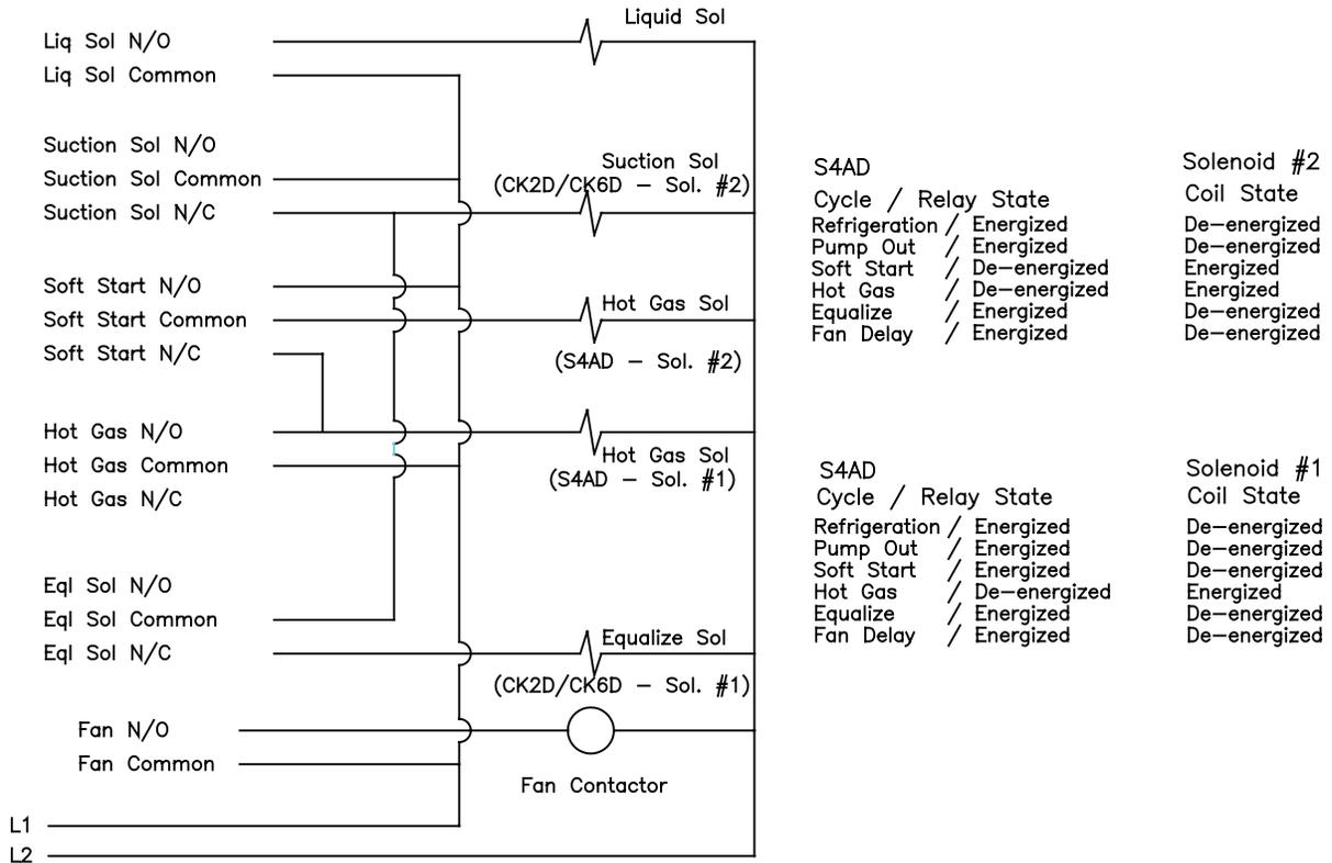
**Note:** The above wiring diagram is to be used only for a R/S defrost controller. If other manufacturer's controller is used, please consult their electrical diagram
