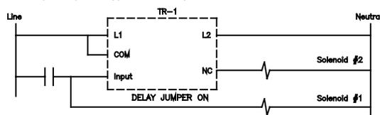
Valve Sequencing - Stepped on Opening & Closing
